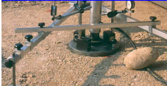
Static load plate test
