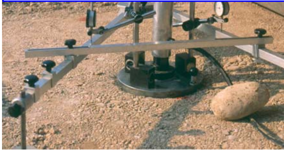
Static load plate test
