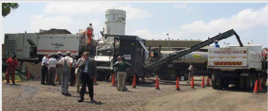
Recycling production of 200 t/h with cement and foam
