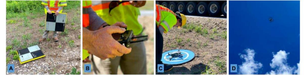
Figure 3. UAS thermal imaging set up on I-69 (A: Placing GCPs, B,C: Pilot flying the UAS, D: UAS flying at about 24m (80 ft)).
