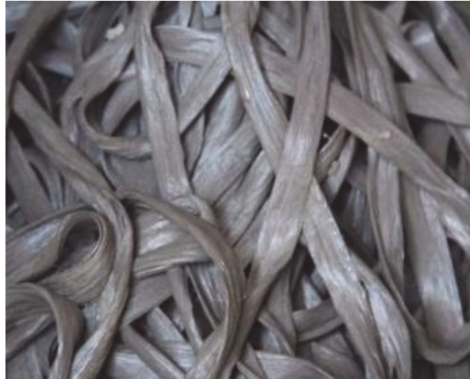
Fig. 11. Photo of formable reinforcement just after production (Balázs, Sólyom, 2023)
