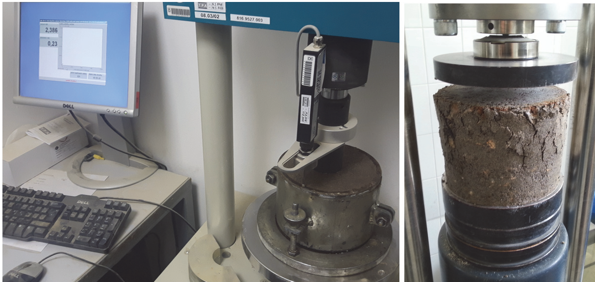
Fig. 1. Test specimens (left – IBI test; right – compressive strength test)
