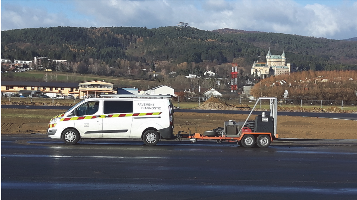
Fig. 5. FWD measurement ("Prievidza" Airport)
