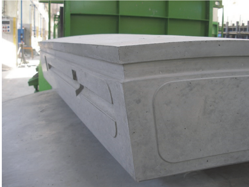
Fig. 6. Precise shape of the segment with a gutter for glued sealing of joints
