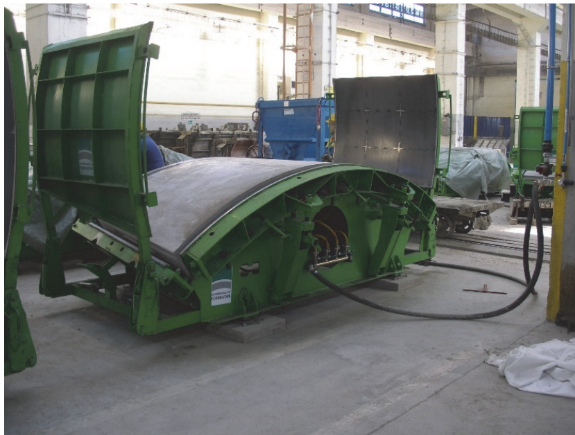
Fig. 5. Mould for production of segments of the Prague subway
