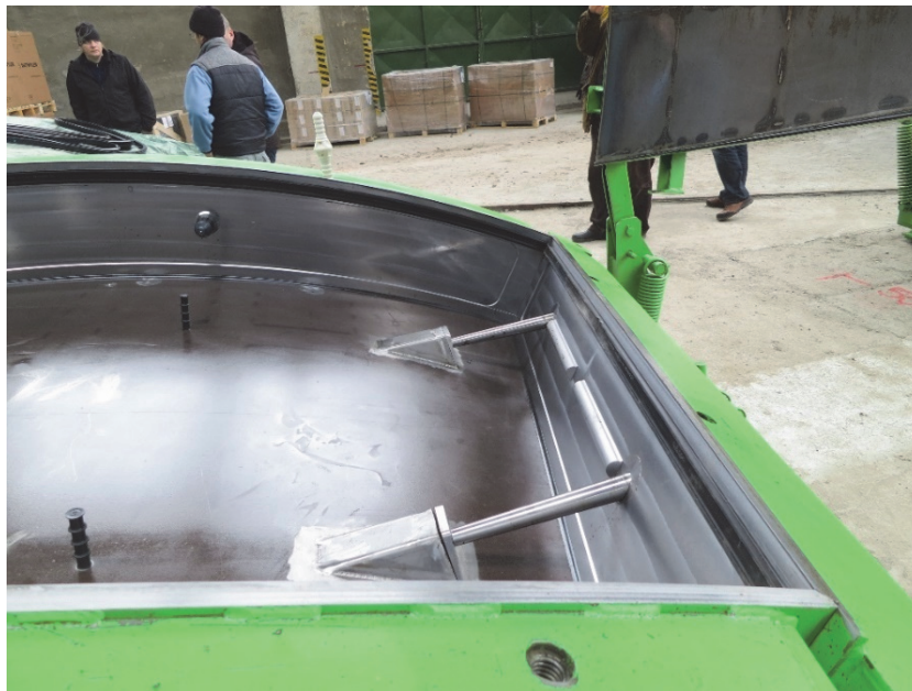
Fig. 7. Detail of the steel mould with glued rubber sealing
