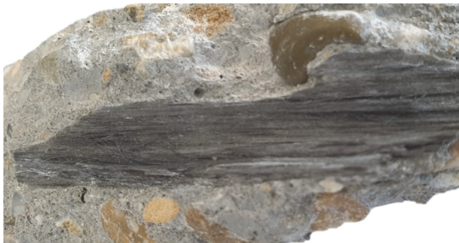
Fig. 12. The bond of formable reinforcement in direct contact to concrete creates an excessive bond (Balázs, Csurgai, Sólyom, 2022)
