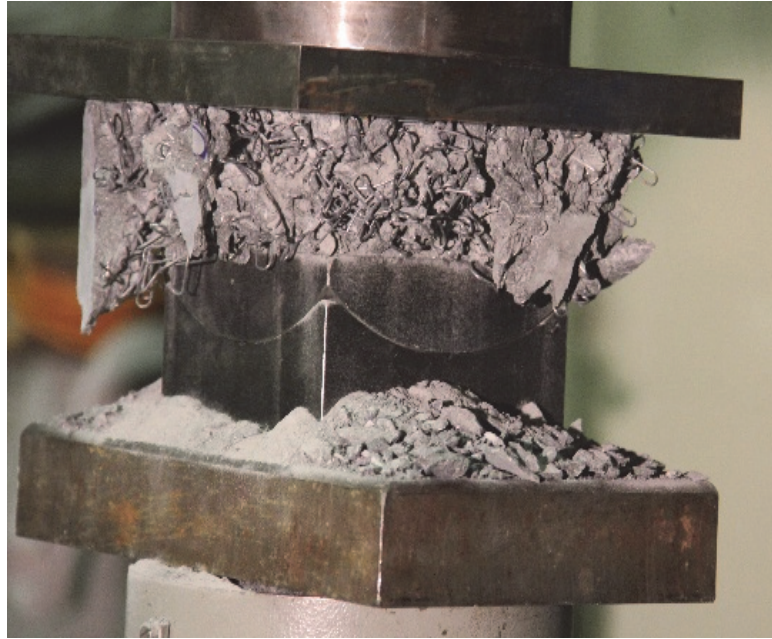
Fig. 14. Extraordinary strain of SIFCON including three dimensional fibres (PERFYCON) in compression
