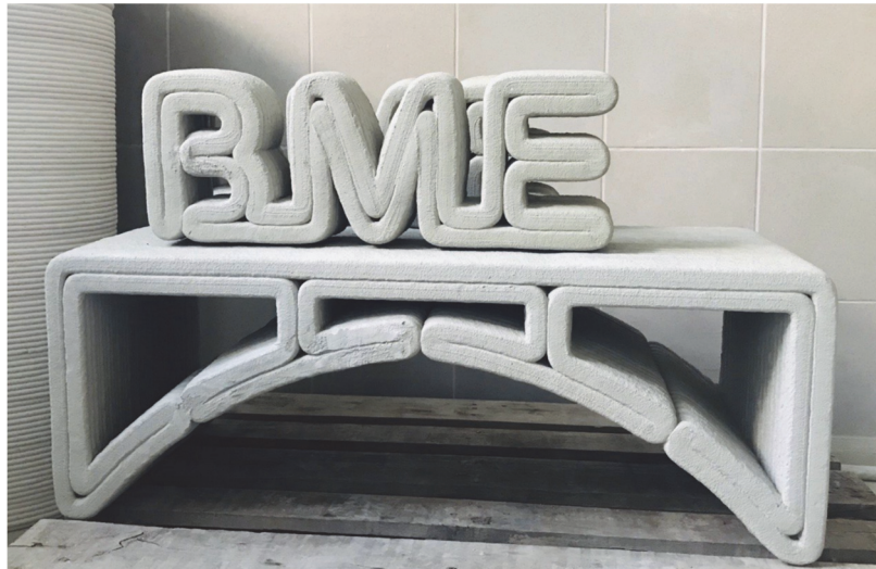
Fig. 2. First bridge in Hungary produced by 3D concrete printer (Budapest University of Technology and Economics, Laboratory of Department of Construction Materials and Technologies)
