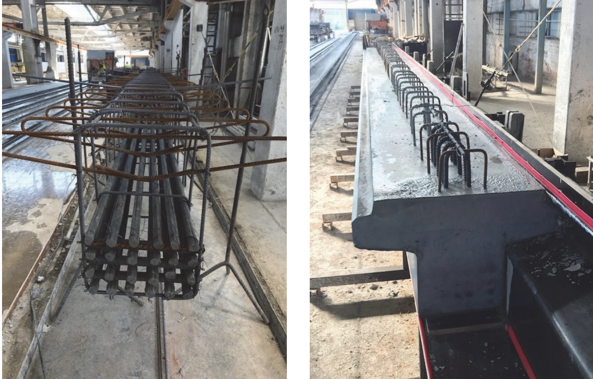
Fig. 13. Bridge girder with CFCM reinforcement (Balázs, Sólyom, 2021)
