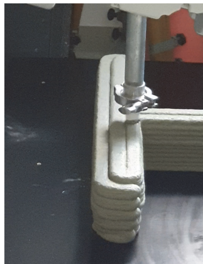
Fig. 3. Concept of printed segments of a bridge in 3D concrete printing that are joined by reinforcement and infill concrete (Budapest University of Technology and Economics, Laboratory of Department of Construction Materials and Technologies)
